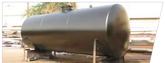
UNDER GROUND FUEL STORAGE TANK
